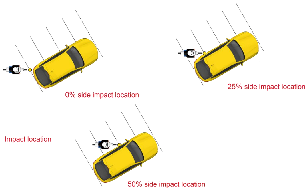
Figure 1-6 Impact Locations for Car-to-Motorcyclist Overtaking
