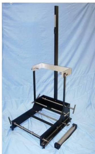
Figure 24: HPM Calibration Jig (GLORIA)
