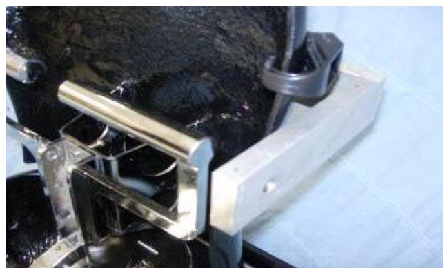
Figure 26: HPM back pan held by retaining strap.
