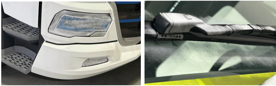
Figure 2-4 Examples of scanning spray used on reflective surfaces
