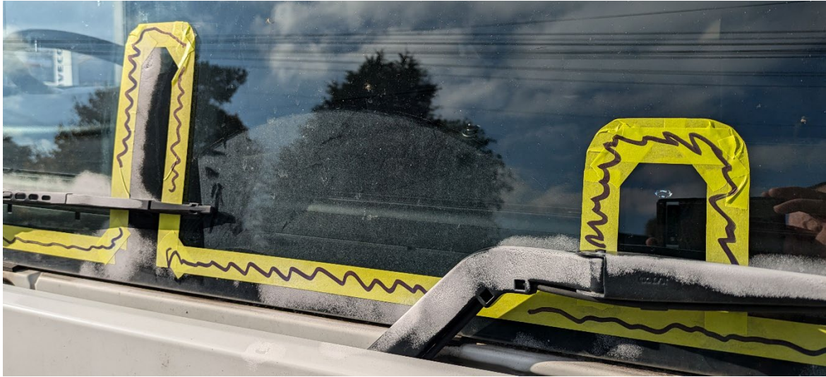
Figure 2-2 Example of tape to outline windscreen sensor
