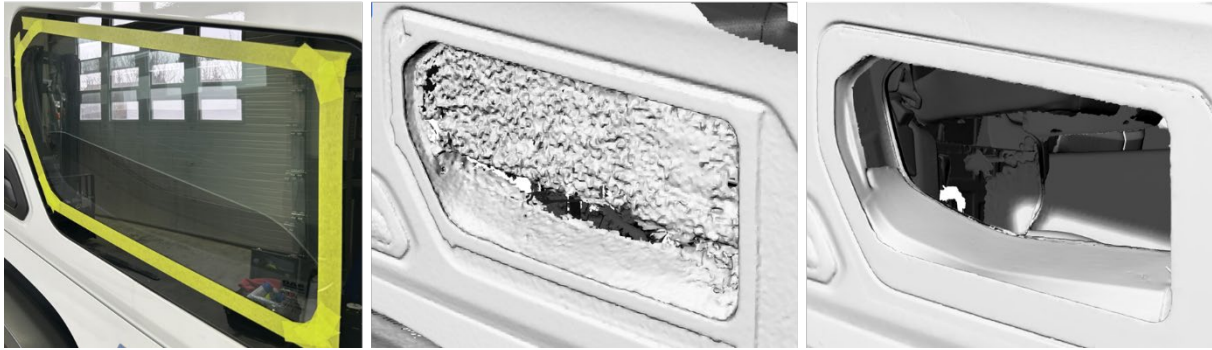
Figure 2-7 Example of vehicle window(left), original scan data (middle) and the model processed to produce a clean outline of the opening (right)
