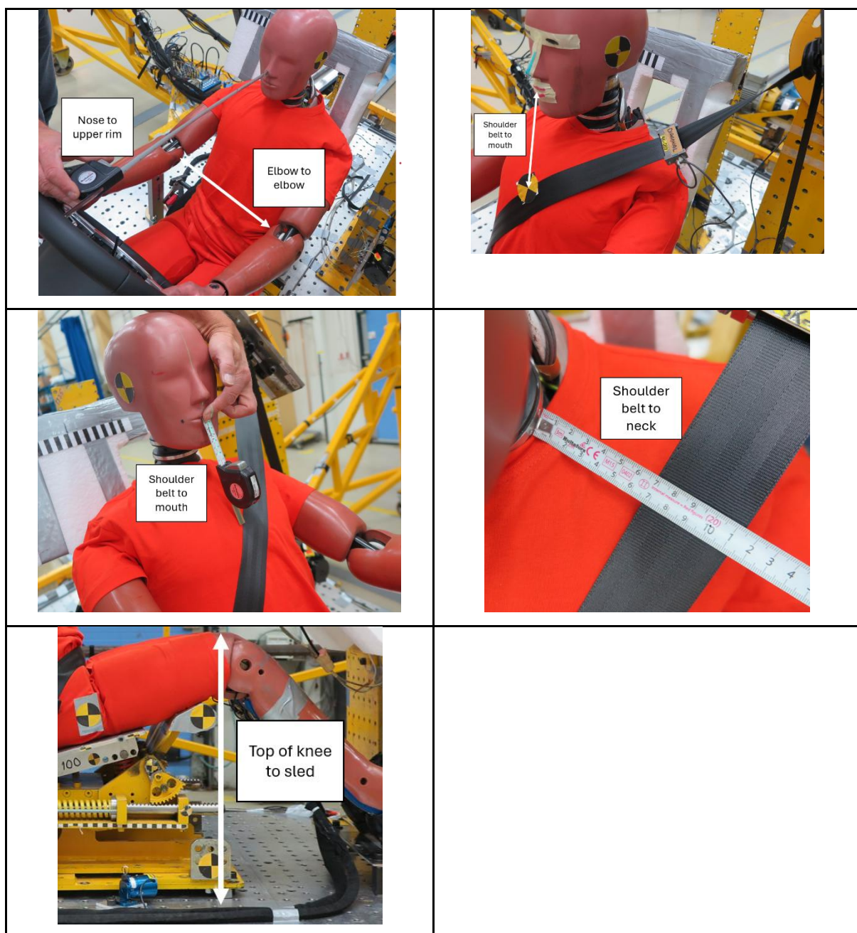
Figure 11: Nose to Rim, Elbow-to-Elbow, Shoulder belt to Mouth, Shoulder Belt to Neck and Top of Knee to Sled Measurements
