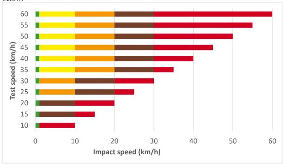
To aid understanding, the following table illustrates the speed range for each colour at a test speed of 60km/h.
