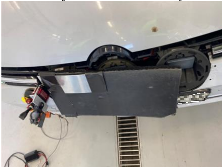
Figure 6 UTAC Electronic Servo Blocking Method
