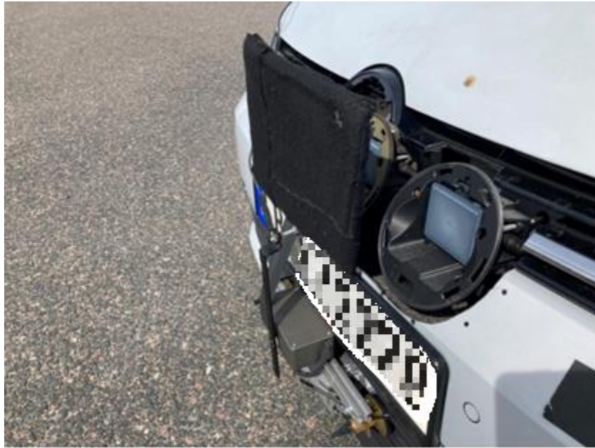
Figure 7 IDIADA Electronic Servo Blocking Method
