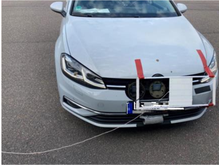
Figure 5 Thatcham Research Manual Blocking Method
