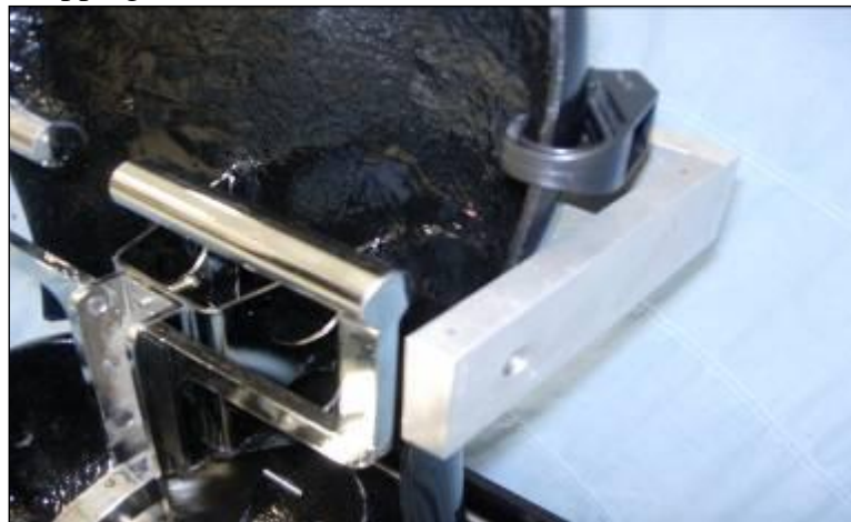
Figure 4. H-PM back pan held by retaining strap
